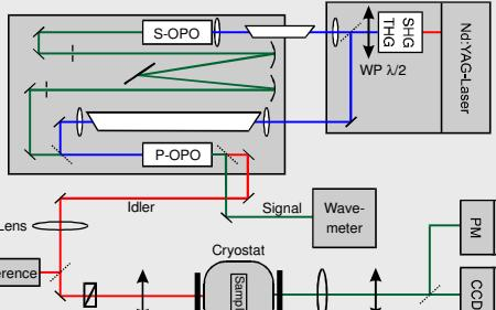
SHG/THG: second/third harmonic generation, OPO: optical parametric oscillator, S/P-OPO: seed/power OPO, WP: waveplate, PM: photomultiplier, CCD: camera, PC: computer
